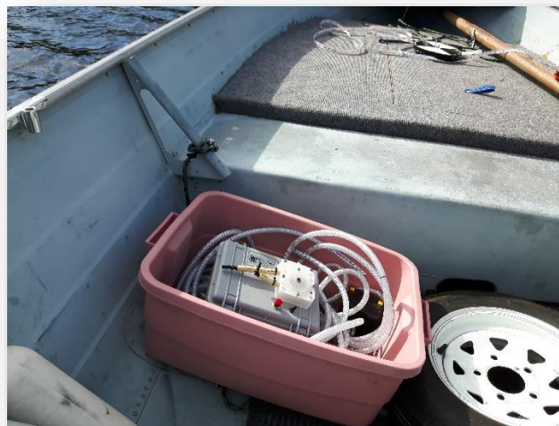
pump to sample bottom waters
